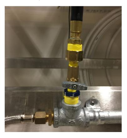
½" NPT M/F conversions on either side of a ¼" NPT needle valve
